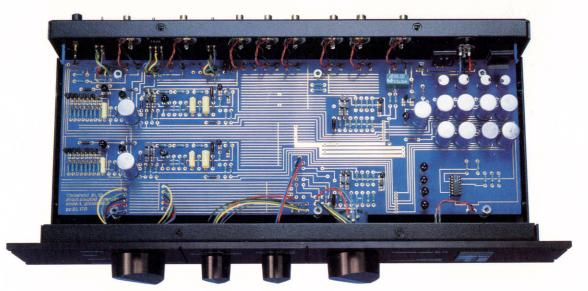
eight transistors per channel, *directly coupled to the input and operated without feedback*, the SL10 circuit forms the active synthesis of a transformer while avoiding the reactance effects that compromise transformer performance. The circuit is a system of such accuracy that it does not require frequency compensation or corrective feedback and therefore maintains extremely high levels of speed and phase integrity.
