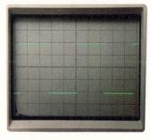
The superiority of DC response capability is clearly illustrated in the oscilloscope display above. Shown is the performance of the SL10 basic circuit reproducing a one-half Hertz square wave. Note the total absence of sag and, thereby, the capability for unencumbered low frequency performance.
